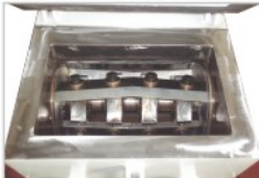
平型机室 Crushing chamber of Flat
